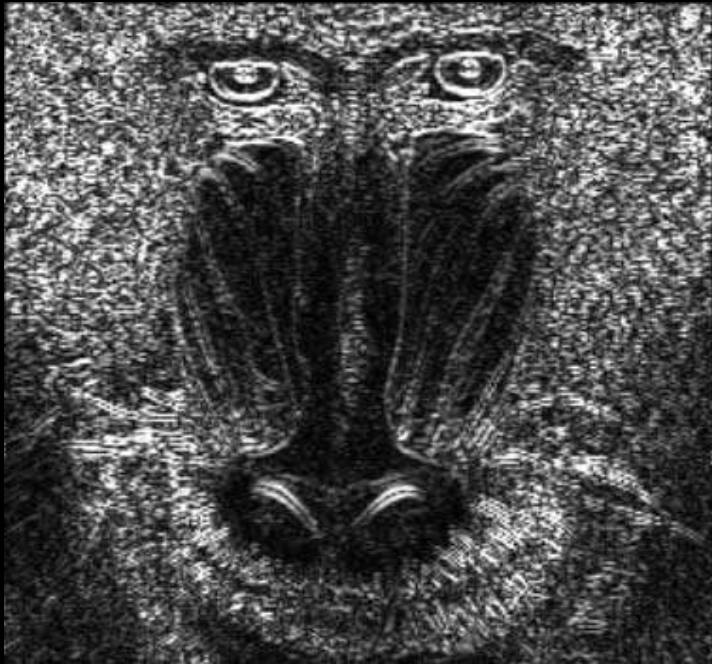
Sobel edge detection on gray Mandrill image
