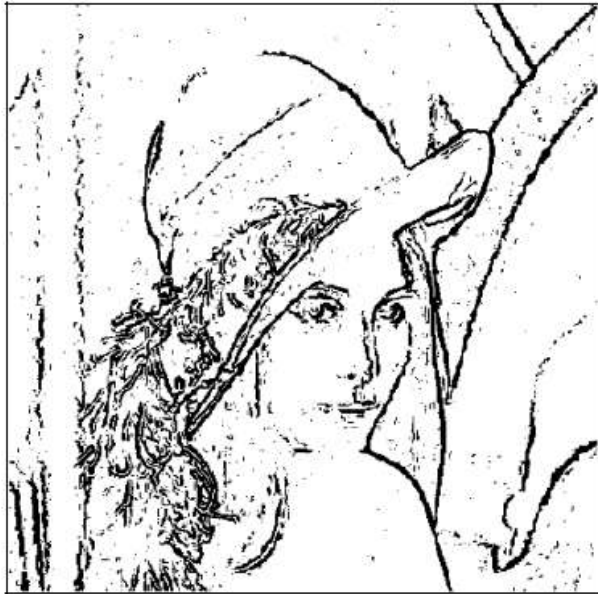
Fig. 12. DV_mean detector: edges of the noised image 'Lena'
