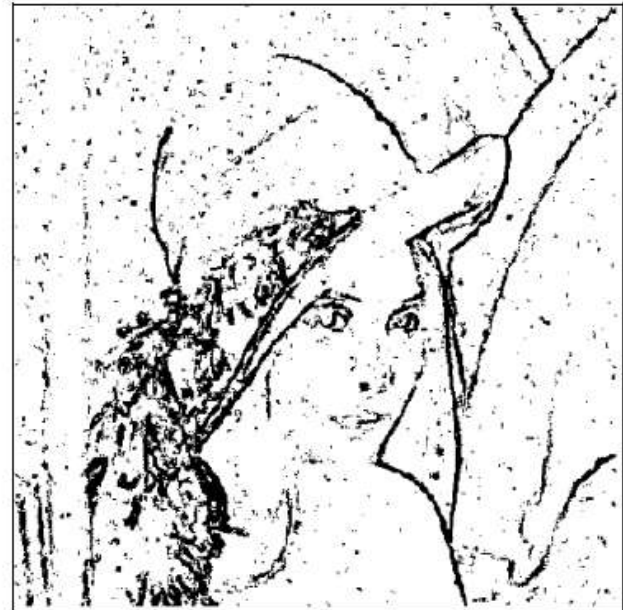
Fig. 10. NNMVD detector: edges of the noised image 'Lena'
