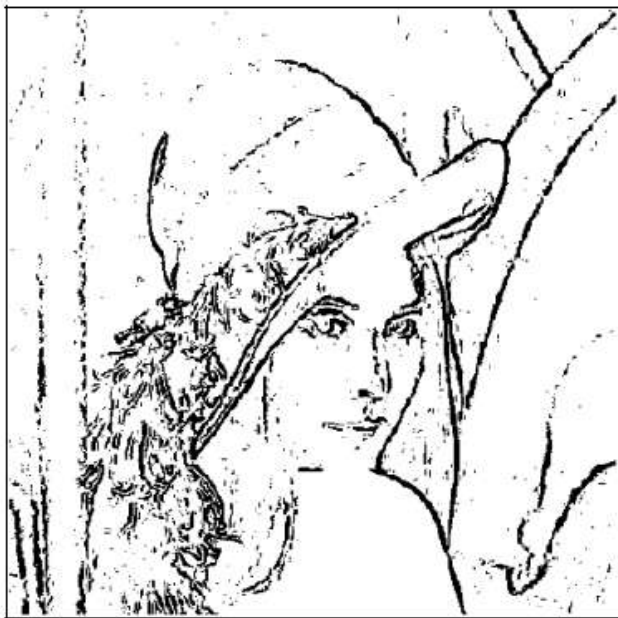
Fig. 16. DV_hv mean detector: edges of the noised image 'Lena'
