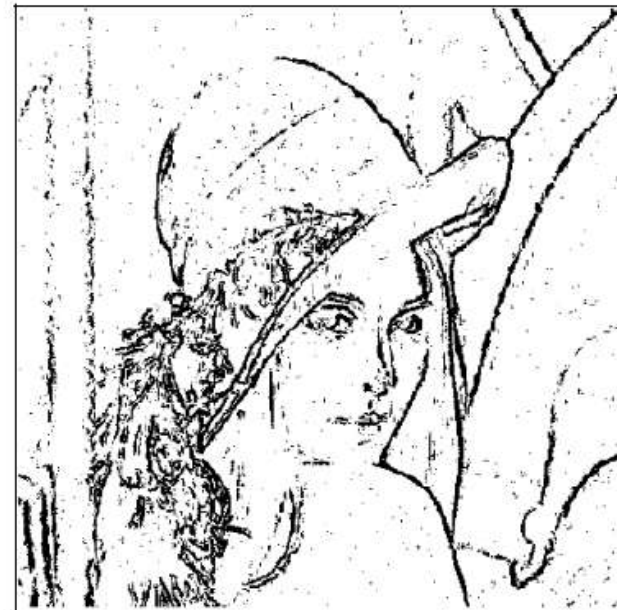
Fig. 15. DV_hv detector: edges of the noised image 'Lena'
